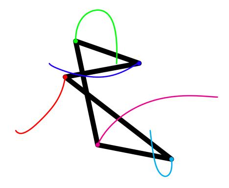
(Example for possible joint trajectories of a five-bar linkage.)
